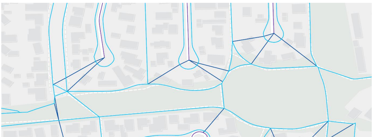
Figure 25: Example of misplaced connectors issue – here the network gives a possible path to exit these cul-de-sacs when this is not possible on the ground. This is mitigated by a low speed on connectors, so the time to use the unphysical connector path is increased to be similar to going around. Here the connectivity layer (dark blue) gives a possible path between the roads (purple) within the cul-de-sacs and the footpaths (light blue) in the park,
